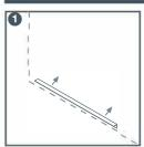
The L profile piece that you will find in the lower unit box is fixed to the wall and should be adjusted.
