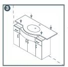
Ceramic, glass or marble bench is put on the adjusted unit. Ceramic Washbasin should be fixed on the wall with connecting fittings.
