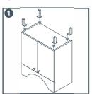
The feet that are in the accessories bag will be fixed to lower unit with 3 5x20 screws
