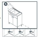
Bench is fixed on the wall with silicone, and for 24 hours it should not be moved and should not be wet.
