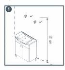
Upper unit hanging part holes will be inserted with 8 mm nails according to hanging height. Просверлите отверстия
