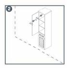
Hanging equipment is fixed on the body of the side cabinet. The side cabinet is placed onto the adjusted L profile and then should be fixed to the wall. Подвесные детали крепятся к корпусу шкафа; затем шкаф необходимо
